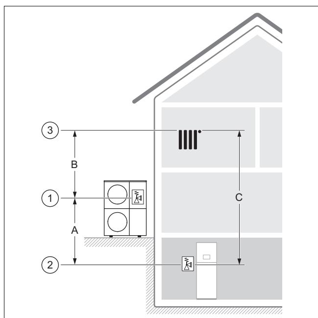
The position (1) of the expansion relief valve in the outdoor unit, the position (2) of the expansion relief valve in the heating circuit, and the position (3) of the highest point in the heating circuit are relevant here.
