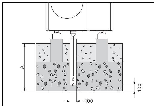
For a region with ground frost, dimension A is  $\geq 900$  mm and, for a region without ground frost, it is  $\geq 600$  mm.
