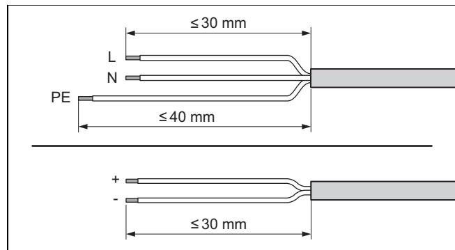
2. Strip the electrical wire as shown in the figure. In doing so, ensure that the insulation on the individual conductors is not damaged.
