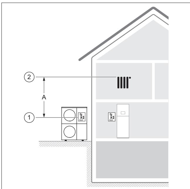
The position (1) of the expansion relief valve in the outdoor unit and the position (2) of the highest point in the heating circuit are relevant here.
