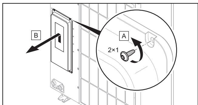
1. Note that the cover contains a safety-relevant seal which must be effective in the case of a leak in the refrigerant circuit.
