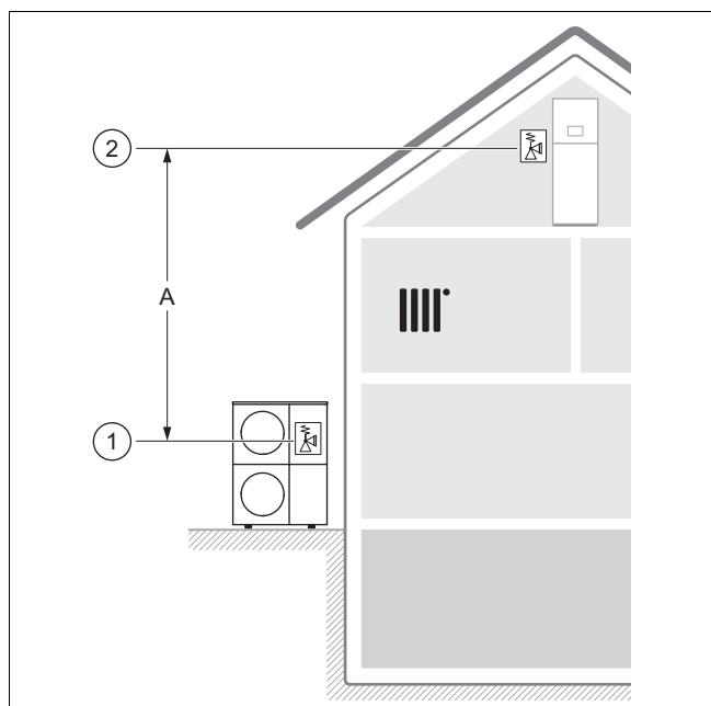
The position (1) of the expansion relief valve in the outdoor unit and the position (2) of the expansion relief valve in the heating circuit are relevant here.
