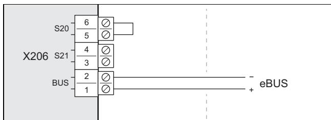
3. Connect the eBUS line to connection X206, BUS.
